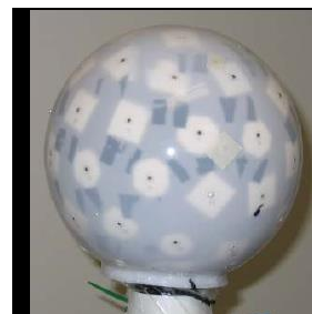
Spherical microphone array
