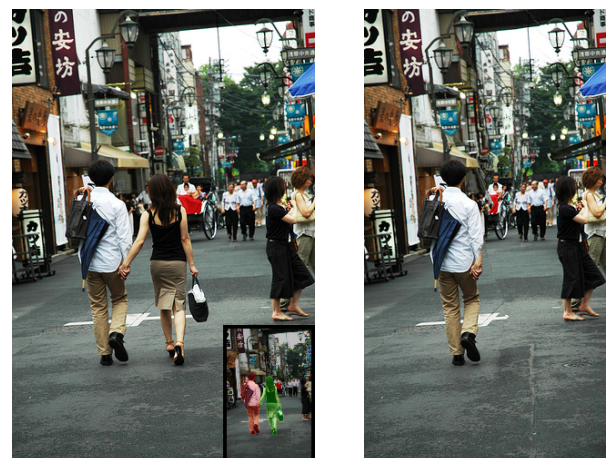
Figure 11: Simple object removal: the user marks a region for removal (green), and possibly a region to protect (red), on the original image (see inset in left image). On the right image, consecutive vertical seam were removed until no 'green' pixels were left.
