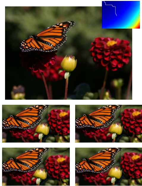
Figure 7: Optimal order retargeting: On the top is the original image and its transport map \mathbf{T} . Given a target size, we follow the optimal path (white path on \mathbf{T} ) to obtain the retargeted image (top row, right). For comparison we show retargeting results by alternating between horizontal and vertical seam removal (top row, left), removing vertical seams first (bottom row, left), and removing horizontal seams first (bottom row, right)
