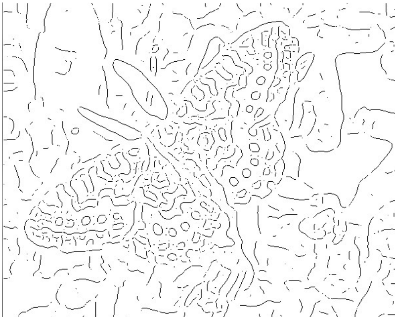
Thresholding gradient with a lower threshold
