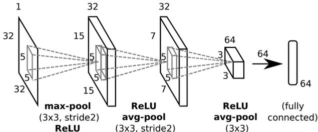
Figure 2. KITTI  $\mathbf{z}_\theta$  architecture producing  $D = 64$ -dim. features: 3 convolution layers and a fully connected feature layer (non-linear operations specified along the bottom).
