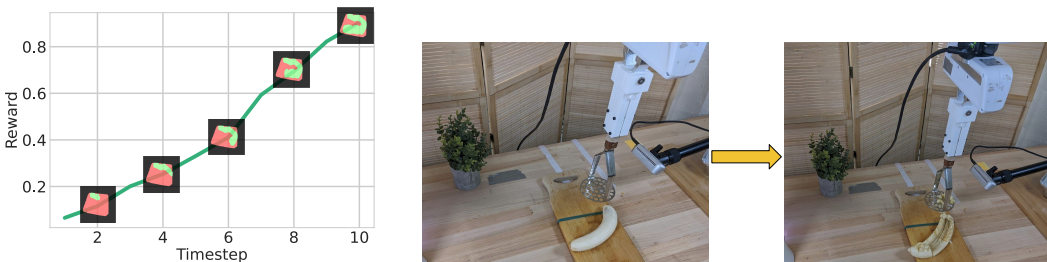
Figure 4: Left: Progress of SPARTA’s reward in a typical training episode; overlaid SPOC [9] affordance maps show how SPARTA continuously transforms actionable regions during an episode. Right: Policy trained on spreading ketchup on bread is able to transfer to smashing banana.
