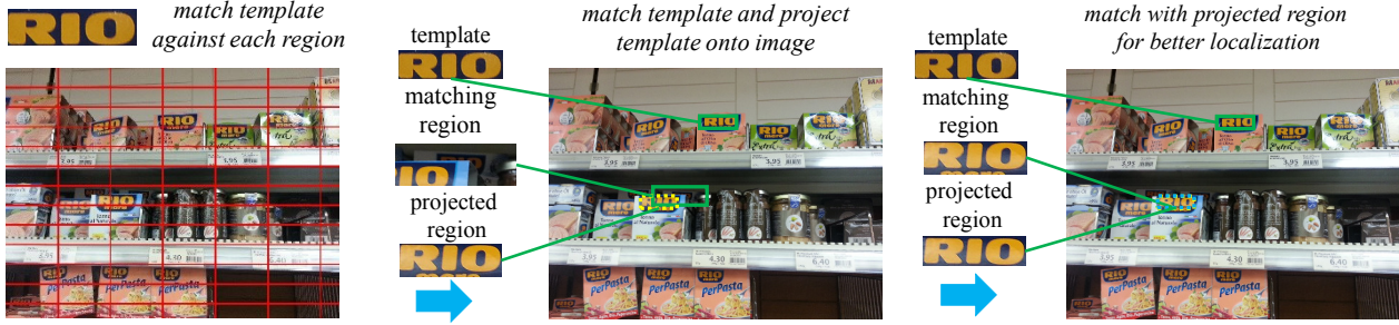
Figure 3. Overview of the matching step. We divide the image into grid cells and match local features from a cluster’s representative text box (the “template”) with those in each of the grid cells (left). For each matching, we project the template onto the image (middle). Then we refine the text box localization by matching the template with the projected region (right). See Sec. 3.2.2.
